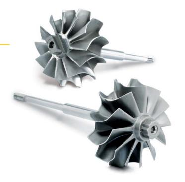
The assembly of the shaft and turbine is a welded combination of two materials (steel and INCONEL®) providing toughness for the shaft and high operating temperatures (up to 1000 °C) for the turbine.
